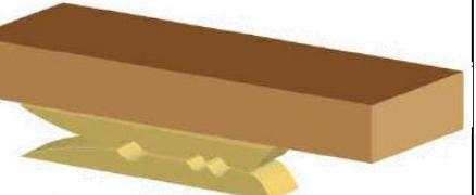
Check the peg holes are large enough to allow axles to move freely.
